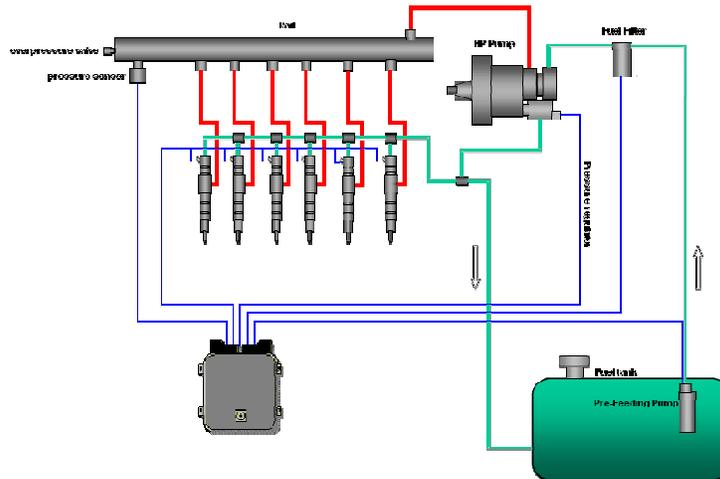
The Marine common rail ecu is an ECU for Common Rail Diesel engines with up to 6 cylinders. It is developed for use in combination with solenoid or piezo injectors. The software is provided with an optimized function range. The ECU is able to operate in a 12 V system.
